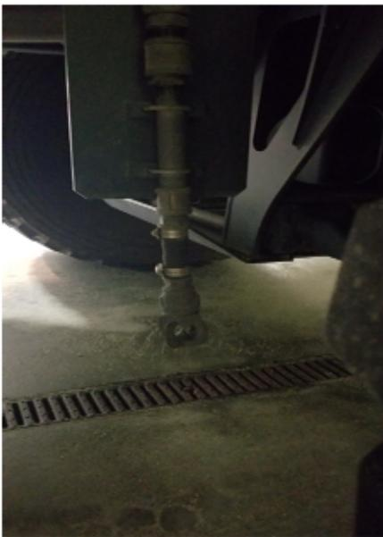
8 under chassis nozzles will flood under the truck with foam to protect it if needed.
