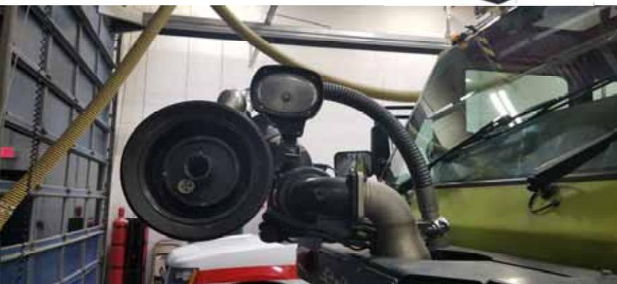
This nozzle can blast foam or 500lb of dry chemicals to deal with “3D fires” - like fuel dripping from a wing that cannot be smothered by foam.
