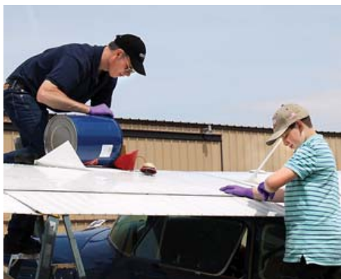
Ross McCurdy of Smithfield, R.I., adds fuel to the airplane he and his son, Aedan, flew 5,000 miles using aviation biofuel made from Camelina plant seed oil. TD Photo ~ Gretchen Hunt
